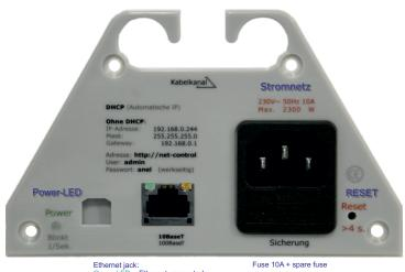
Ethernet jack: Green LED = Ethernet connected Orange LED = Data transmission
